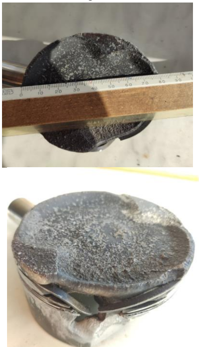
Fig. 1. Wear of the working surfaces of the piston group as a result of detonation
